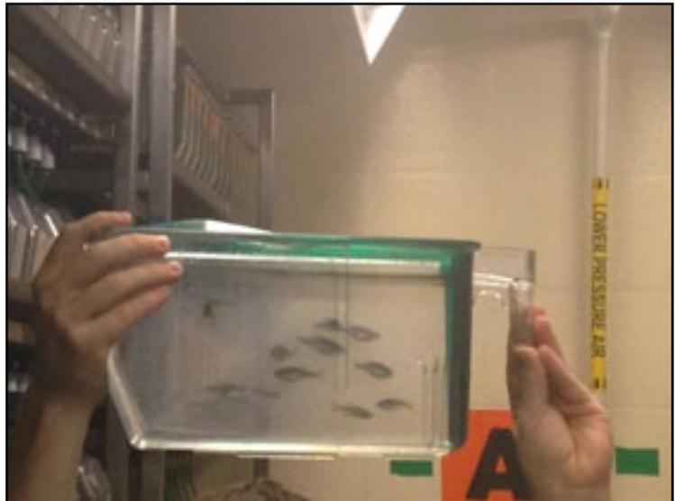
The polycarbonate tanks, by [Aquaneeering](#), are designed for efficient operation and maintenance and can be autoclaved for sterilization.
