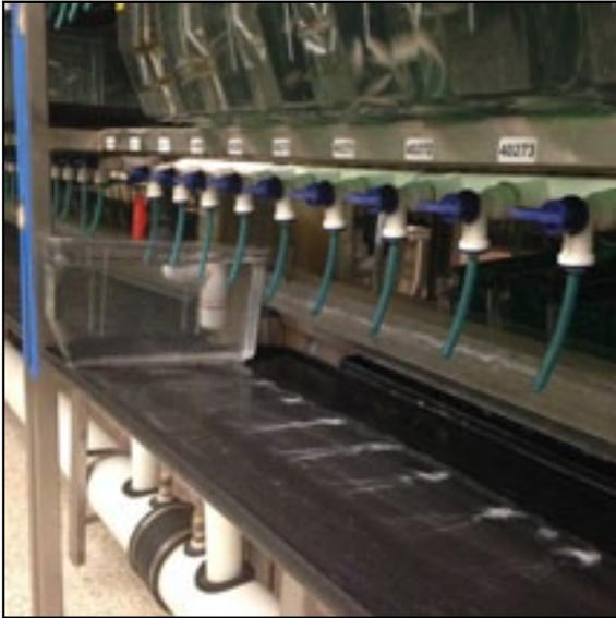
Water drips from the plastic tubes and overflows out the back into a collection gutter, achieving a 12% daily water change.
